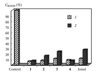
**Fig. 6.** Antioxidant activities of phenols **1—4** in the accumulation of hydroperoxides ROOH during the oxidation of oleic acid at 50 (*I*) and 65 °C (*2*). The oxidation duration is 4 h; the concentrations of the additives are  $10^{-3}$  mol L<sup>-1</sup>. The ROOH content in the oxidation of oleic acid without additives (blank experiment) was taken as 100%.
