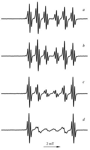
Fig. 3. Temperature dependence of the ESR spectra of radical 3, T/K: 200 (a), 220 (b), 250 (c), and 270 K (d).
