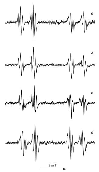
Fig. 1. Temperature dependence of the ESR spectra of radical  $1^{\circ}$ , T/K: 210 (a), 240 (b), 280 (c), and 300 (d).
