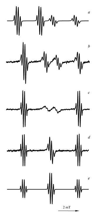
Fig. 2. Temperature dependence of the ESR spectra of radical  $2^{+}$ : simulated spectra for  $2A^{+}$  at 200 (a) and 300 K (e) and experimental spectra (b-d) at 200 (b), 240 (c), and 300 K (d).
